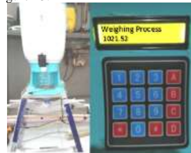
Figure 23. The sugar weighing process can be seen via the LCD screen.
