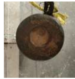
Figure 16. Provide a load of 1kg during the calibration process.
