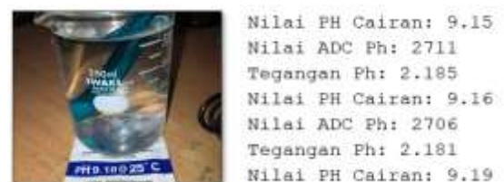
Figure 8. Calibration of The Buffer Solution pH 9.18
