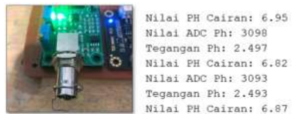
Figure 7. pH Sensor Calibration
