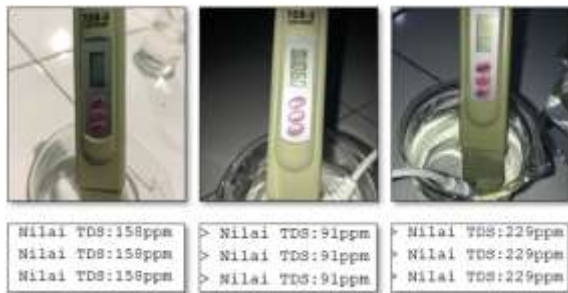
Figure 6. TDS Sensor Test Result
