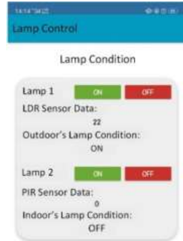
Figure 11 The results of the PIR and LDR sensors display in the lamp control menu
