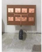
Figure 12. Rectangular microstrip antenna H-Slot array 2x4 front view
