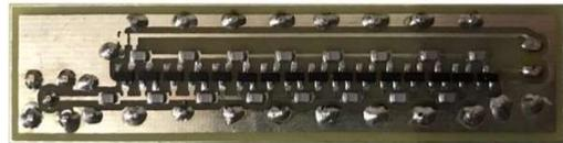
Figure 13. Fabrication of 8-stage rectifier voltage doubler circuit
