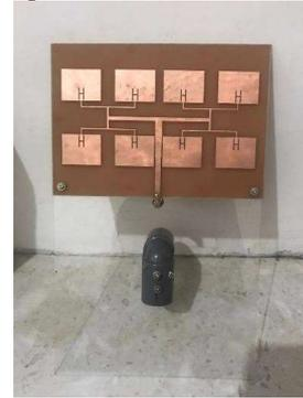
Figure 12. Rectangular microstrip antenna H-Slot array 2x4 front view
