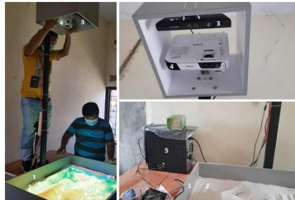
Figure 2. Interactive sand table complete overview; 1: sand box; 2: beach sand; 3: a Microsoft Kinect 360 camera; 4: an Epson EB-e500 projector; 5: a desktop computer; 6: 3D virtual environment
