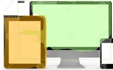
Figure 4. Cellphone image in front of monitor not detected by pretrained data model
