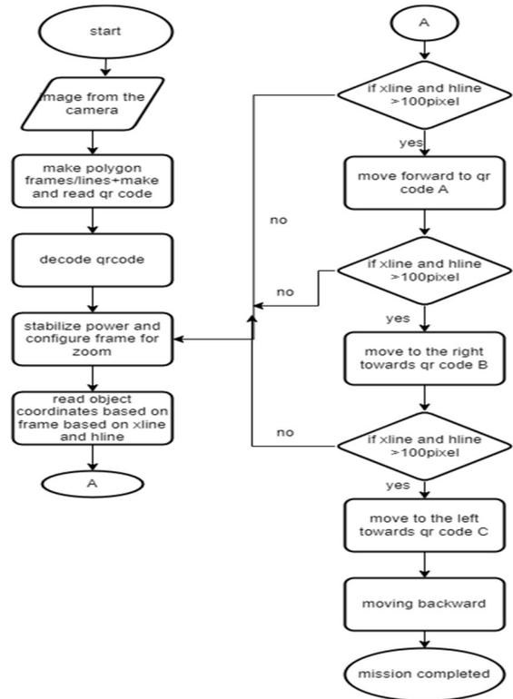
Figure 5 Flowchart Image Processing
