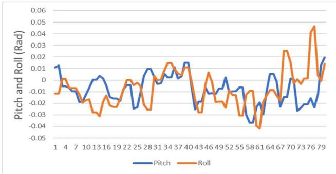
Figure 5. Indoor 150 cm Height Pitch and Roll Motion Chart
