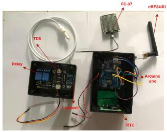
Fig. 7 Circuit on Node Sensor
