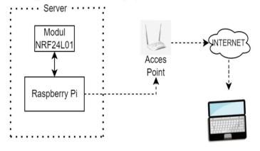
Figure 4. Diagram hardware in node server
