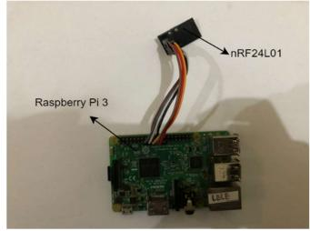
Fig. 6 Circuit on Node Server
