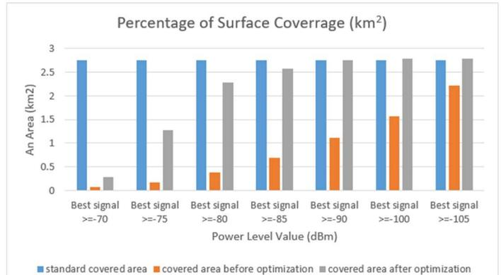
Figure 7. Graph of Surface LTE Network Coverage Percentage Before and After Optimization
