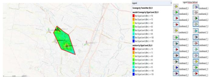
Figure 8. Result of the existing Telkomsel site RSRP value
