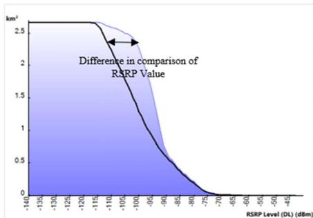
Figure 12. Histogram Graph of Comparison of RSRP Values Before and After Optimization
