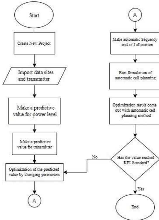
Figure 1. Coverage Modelling Diagram with Automatic Cell Planning Method
