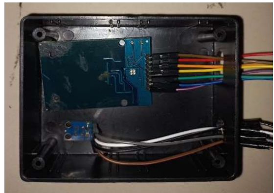
Figure 7. Hardware Implementation of the RFID and MLX614
