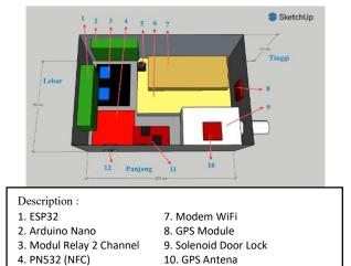
Figure 5. Mechanical Design of Control Box
