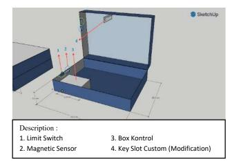
Figure 4. Mechanical Design of Suitcase Implementation Side view is open
