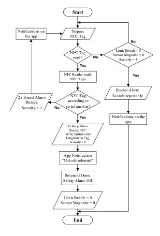
Figure 2. Flowchart Open Security Key
