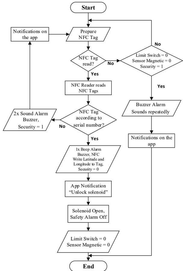
Figure 2. Flowchart Open Security Key
