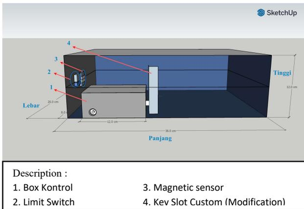
Figure 3. Mechanical Design of Front View Suitcase Implementation
