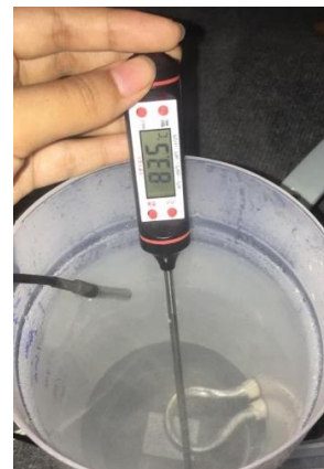
Figure 15. DS18B20 Temperature Sensor and Manual Testing
