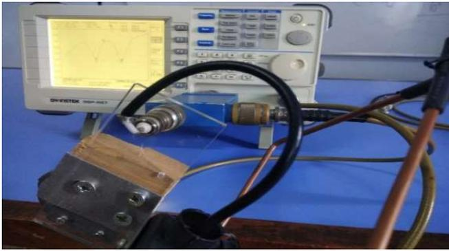
Figure 6 Testing the return loss of a double biquad antenna
