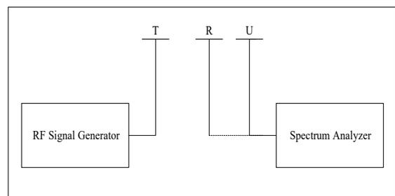
Figure 8. Block Diagram of Antenna Gain Measurement
