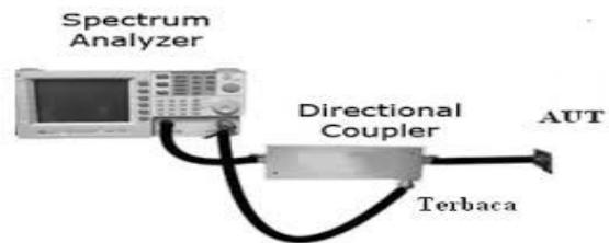
Figure 5. Antenna Return Loss Measurement method
