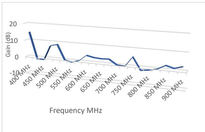
Figure 9. Gain graph of double biquad antenna
