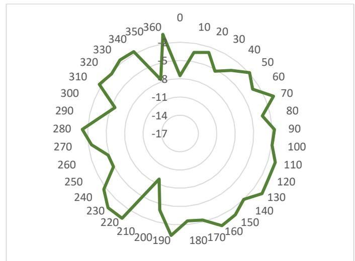
Figure 10. Polar Diagram of the double Biquad Antenna radiation pattern
