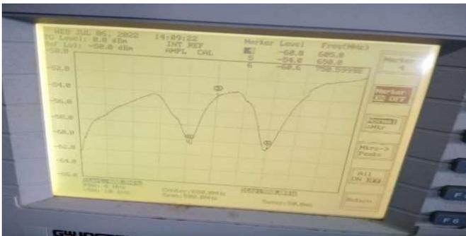
Figure 7. Results of measuring the return loss of a double biquad antenna
