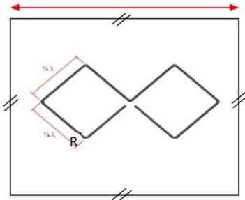
Figure 2 Biquad Antenna Design Size
