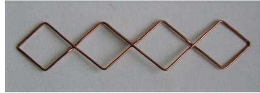
Figure 4. The shape of the double biquad antenna
