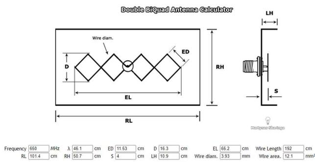
Figure 3. Double biquad antenna design
