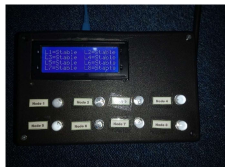
Figure 9. Result Node Server is in Stable state
