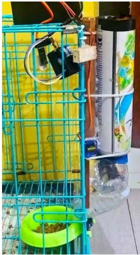
Figure 11. Feed Container System
