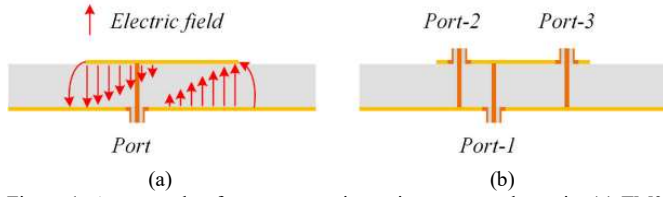
Figure 1. An example of a common microstrip antenna schematic. (a) TM01 mode's electric field. (b) Microstrip-based power divider. [12]
