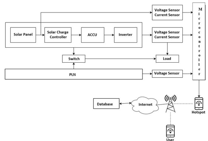
Figure 4. System block diagram
