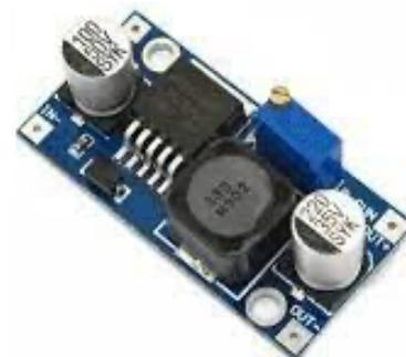
Figure 6. Step Down Module
