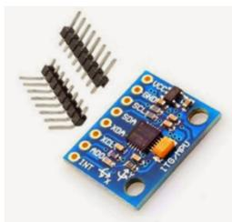
Figure 3. MPU-6050 sensor
