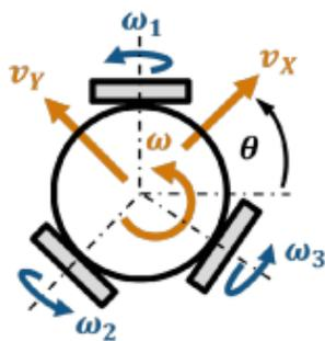
Figure 8. Kinematic OMR
