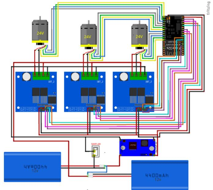
Figure 11. Circuit Electric Robot
