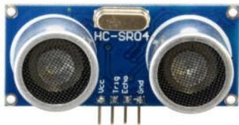
Figure 3. Proximity Sensor with Ultrasonic HC-SR04
