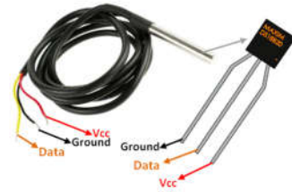
Figure 4. Temperature Sensor (DS18B20)
