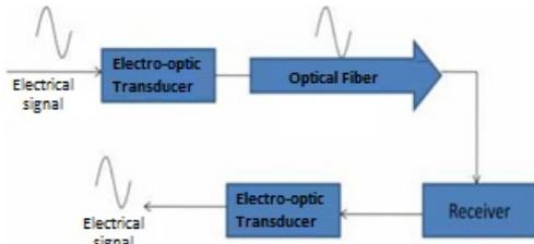
Figure 2. Fiber optic working principle
