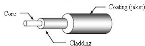
Figure 1. Basic structure of fiber optic
