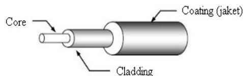
Figure 1. Basic structure of fiber optic
