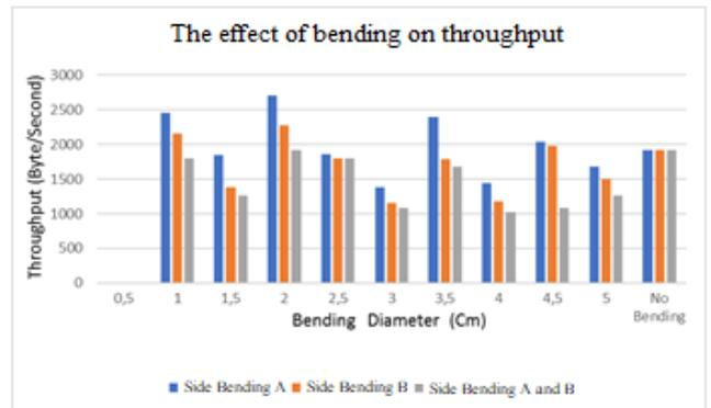
Figure 22. Bending vs Throughput
