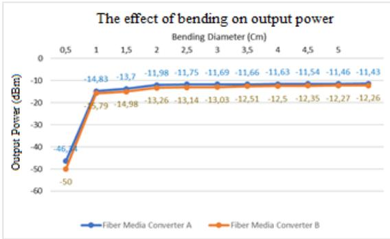
Figure 21. Bending vs power
