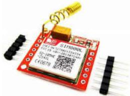
Gambar 6. Modul GSM SIM800L
