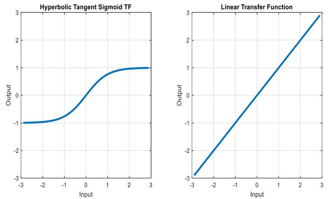
Figure 3. Types of Activation Functions used in the ANN.
