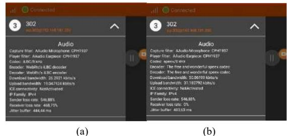
Figure 7. (a) Test of VoIP codec iLBC using softphone linphone; (b) Test Call VoIP codec speex using softphone
