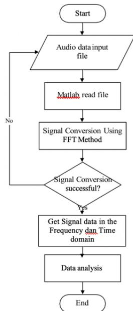
Figure 4. Audio Processing Design Flowchart
