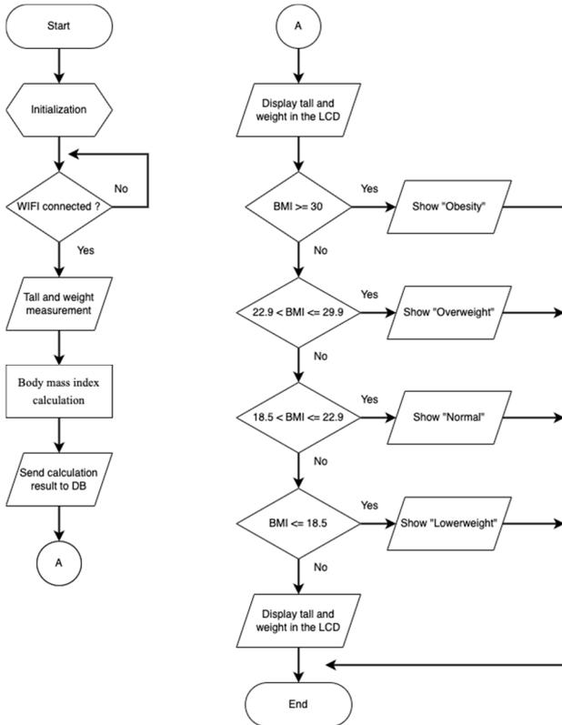
Fig. 2 Flowchart system model
