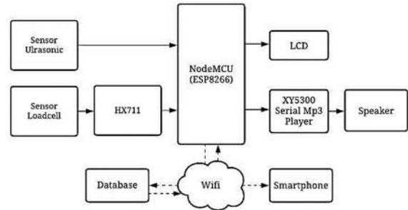
Fig. 1 Diagram block system
